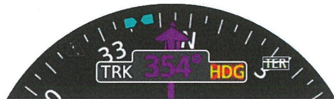
Figure 5- Top of the HSI when HDG failed (with GPS)
