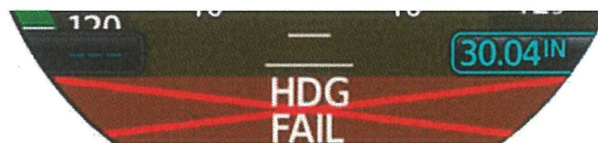
Figure 6- Bottom of the ADI when HDG failed (no GPS)
