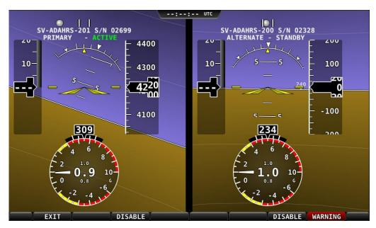
Figure 56 - ADAHRS Cross-Check Comparison
