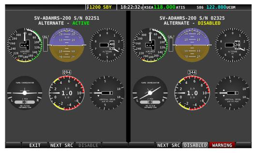
Figure 58 - ADAHRS Cross-Check Comparison - six-pack
