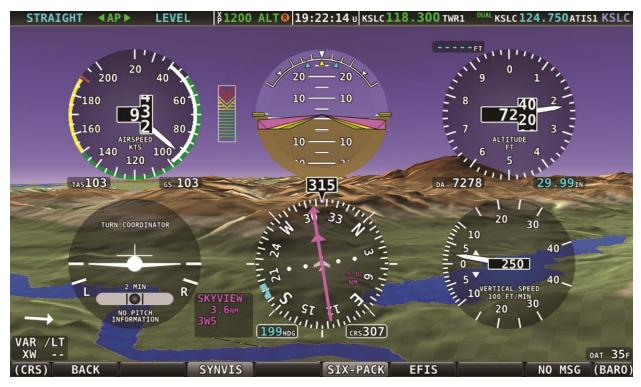
Figure 53 - Analog PFD with Synthetic Vision
