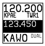
When dual watch is enabled, the SkyView COM Radio monitors the standby frequency for transmissions while simultaneously monitoring the active frequency, allowing you to listen to both (but not simultaneously). This allows you to listen to ATIS on standby, for example, while keeping tower tuned to the active frequency.
