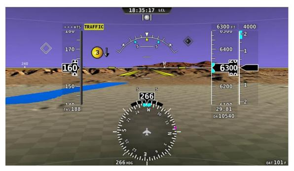
Figure 46 - Traffic Display on Synthetic Vision
