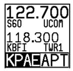
• Press the dual concentric knob on the control panel to load the airport to the control panel (or press APT to cancel your selection):
