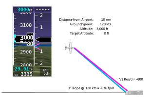
Figure 22 - Vertical Speed Required to Destination
