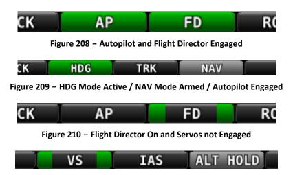
Figure 211 - VS Mode Active / ALT HOLD Mode Armed / Servos Not Engaged
