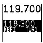
With a valid COM frequency highlighted, (a 25kHz frequency on the SV-COM-C25/X25 and an 8.33kHz on the SV-COM-X83) press the TUNE COM button to send the frequency to the standby frequency:
