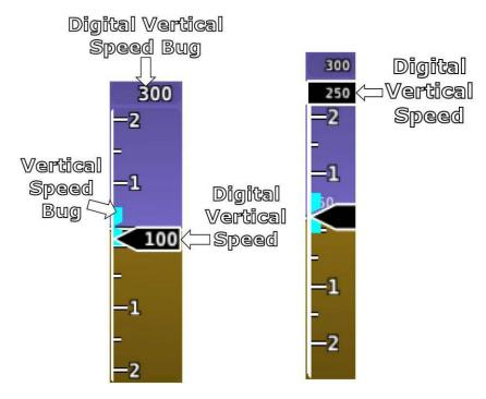
Figure 21 – Example Vertical Speed Indicator.
