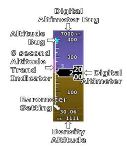
Figure 18 – Example Altimeter
