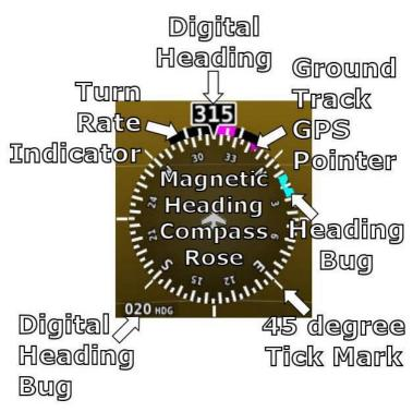
Figure 23 – Example Magnetic Heading Indicator/Directional Gyro
