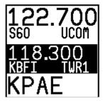
• Use the TWR, ATIS, GND, and ATC buttons to send the associated airport frequencies to the standby frequency location:
