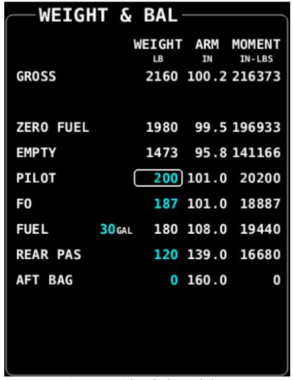
Figure 68 - Weight and Balance Calculator
