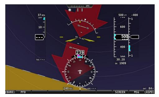
Figure 52 - Extreme Pitch Warning Indicator Arrows
