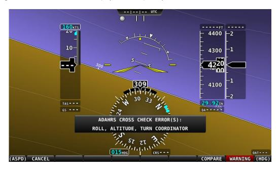
Figure 55 - ADAHRS Cross-Checking Disagreement
