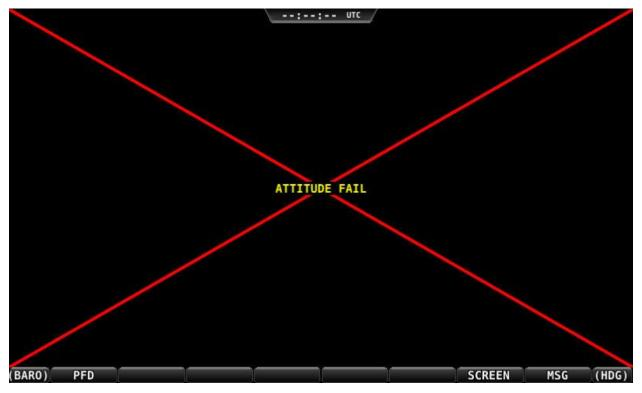
Figure 231 – Example SkyView Failure
