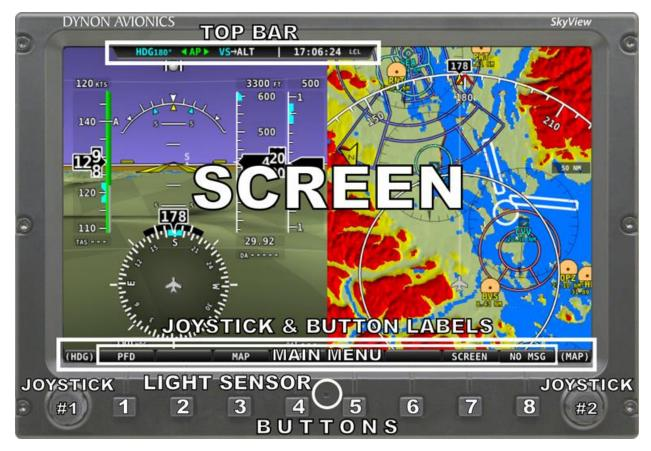
Figure 1-SkyView Display Front Bezel Layout
