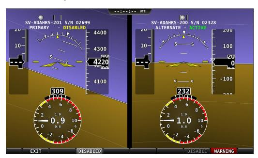
Figure 57 - ADAHRS Cross-Check Comparison (one ADAHRS disabled)
