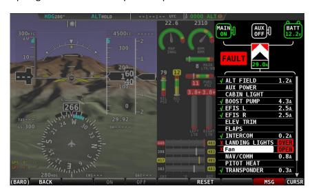
Figure 76 - VP-X Page with Fault
