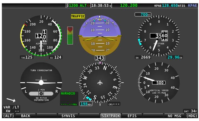
Figure 54 - Analog PFD without Synthetic Vision
