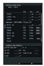
Figure 8-3 Active Flight Plan Page on the MFD
