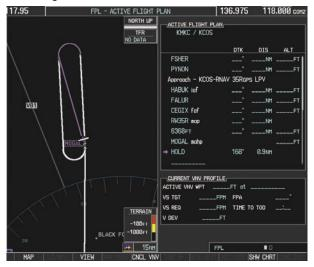
Figure 7-49 Establishing the Holding Pattern
