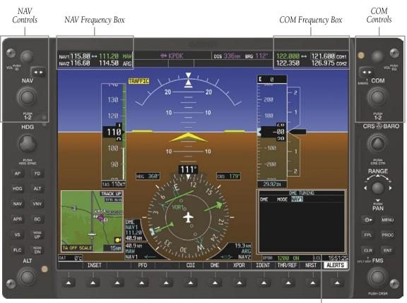
Figure 4-1 G1000 VHF NAV/COM Interface (PFD shown)
