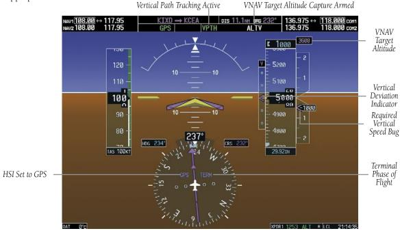
Figure 6-12 Vertical Path Tracking Mode
