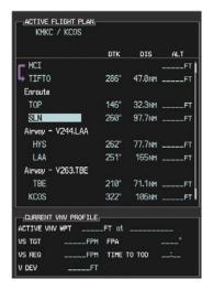
Figure 7-15 TOP Inserted into the Flight Plan
