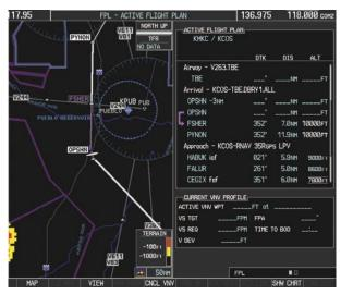
Figure 7-41 Tracking the OPSHN to FSHER Leg
