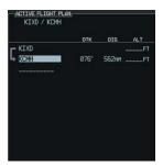
Figure 8-13 Airway Insertion Point
