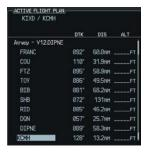
Figure 8-18 Airway Added to Flight Plan
