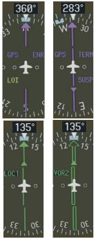
Figure 2-29 GPS LOI, GPS SUSP, LOC1 and VOR2
