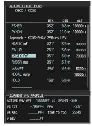
Figure 7-34 Vertical Guidance is Active to the FAF
