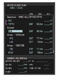
Figure 7-13 Begin Adding V4 to the Flight Plan
