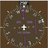
Figure 7-12 Assigned Heading of 290°
